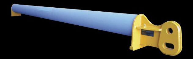
The Maxilug 80 allows users to create their own custom length, medium-lift spreader bar utilizing these heavy duty end units. Designed to accomodate readily available line pipe, Maxirig can supply the units as is or with various pipe lengths to facilitate lift spans from 2 metres up to 13 metres.
