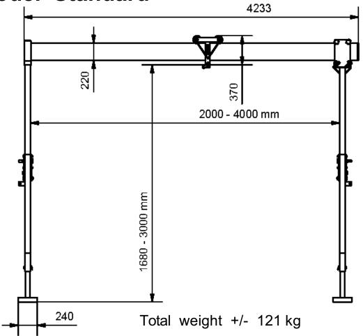
Width of lateral stand 1705 mm Height for hanging the pulley block from 1680 to 3000 mm
